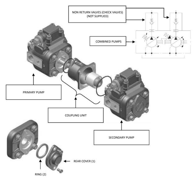
Combined pumps should be mounted in decreasing order of absorbed power, paying attention to the maximum acceptable torques (see diagram on the following page).
