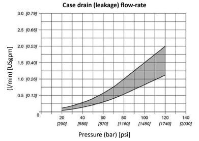
Pump under zero flow setting conditions
